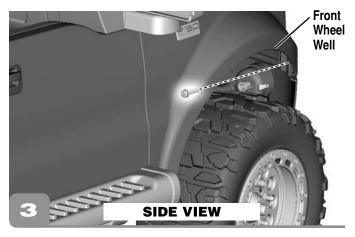
Insert a screw through both front wheel wells and into the front grille. Tighten the screws.
